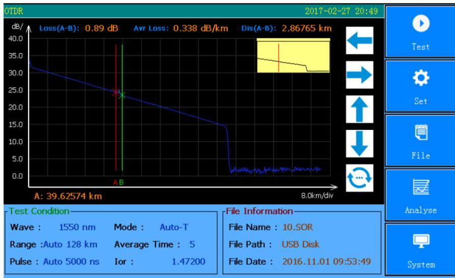
Fig.3-5 Connection Loss Test
