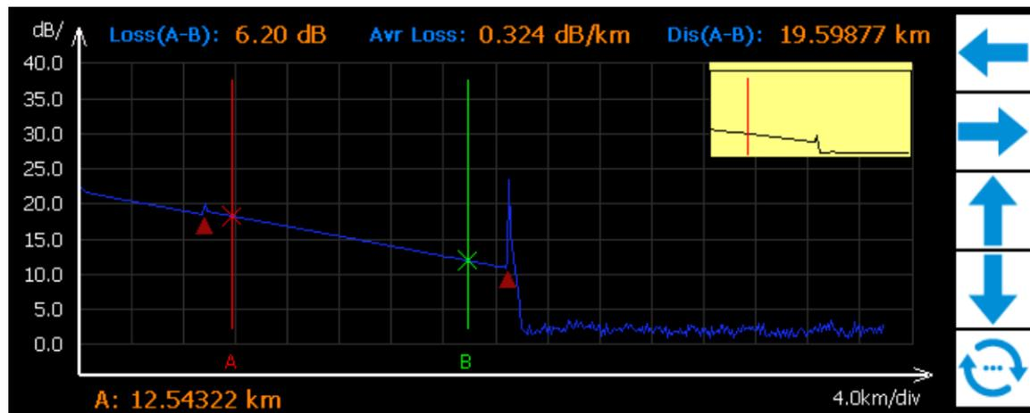
Fig.3-8 Average Loss Measurement
