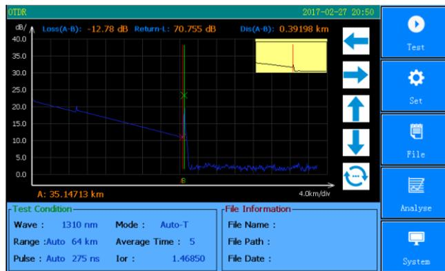
Fig.3-6 Reflection loss test
