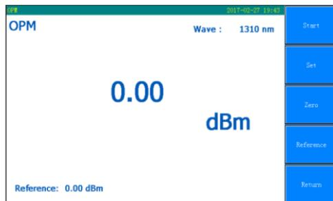
Fig.4-1 Optical power meter test interface
