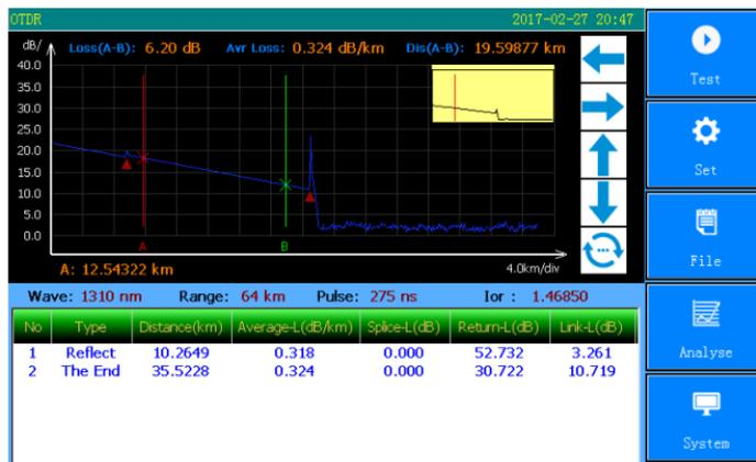
Fig.3-4 Average Loss Test
