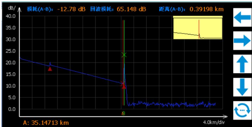
Fig.3-10 Return loss measurement
